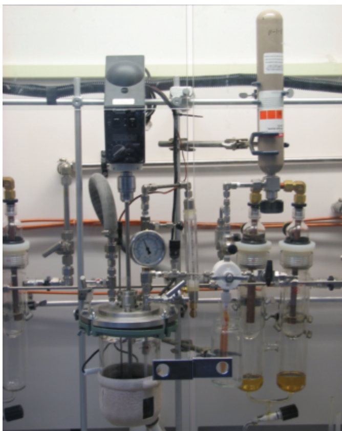
Figure 6 | The ROBO test is run with the laboratory equipment shown. (Courtesy of Evonik RohMax USA, Inc.)
